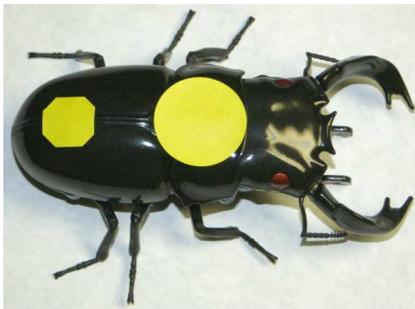
Figure 3: Robotic bug with synthesized vision from an overhead camera and four actuation spaces corresponding to turn left, turn right, move forward, and move backward.
