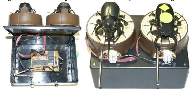
Figure 5: Control interface for the robotic bugs. The interface controls the handheld remote control devices that double as chargers.
