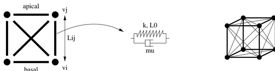
Figure 3: On the left, Odell's model for the simulation of epithelial cells. On the right, extension of the Odell's model to three dimensions.
